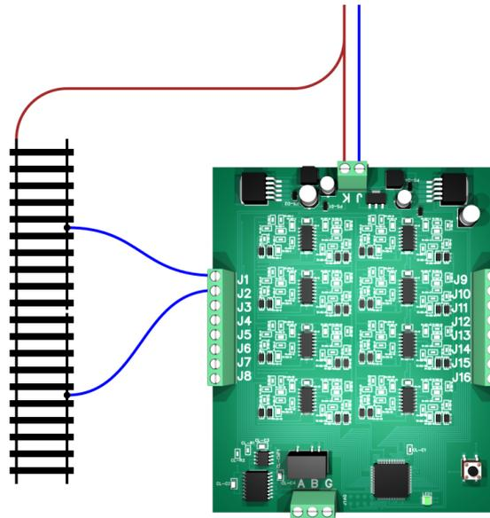
**Warning:** The RailCom™ Reader is rated to 5A. If you have a booster which can produce more than 5A you run the risk of damaging the device in the event of a short circuit. To prevent this either configure the booster to output a maximum of 5A (if possible) or install a DCC circuit breaker between the booster and the RailCom™ Reader.
