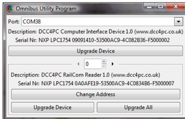
First use the utility program to select your device (address 0 for a new device). The description will help confirm you have the correct device selected. Then click **Change Address**. Change the value next to **Address** to the address you desire for the device: address 1 if this is your first Omnibus device, address 2 for your second, etc.
