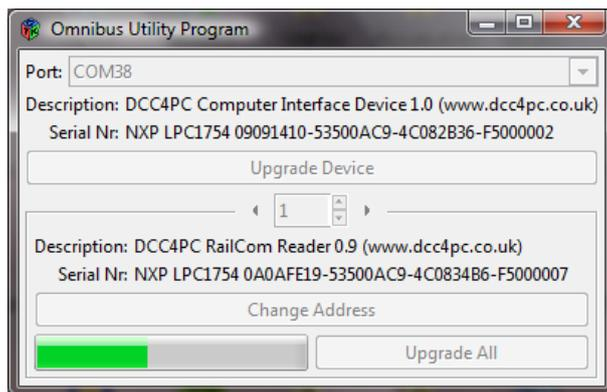
During the upgrade the LED on the RailCom™ Reader will blink red. After the upgrade is complete the LED will turn green and the description of the device provided by the utility program should change to indicate the new firmware version. If the upgrade failed to complete then the LED will remain a solid red.
