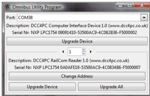
As an alternative, if you have several devices you wish to upgrade, you can click **Upgrade All** instead. This will cause the utility program to search every address from 0 to 255 and, for each device the firmware upgrade is compatible with, upgrade the firmware as described above.
