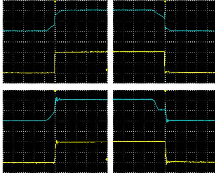
The blue traces show the signals produced by the command stations, while the yellow traces show the signals produced by the cutout device, and sent to the tracks.
